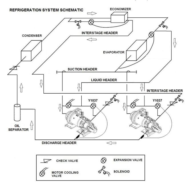
Fig. 15 — Refrigeration System Schematic
