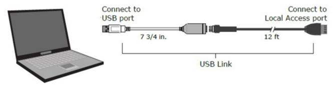
Fig. 29 — Laptop-to-BACview6 Connection Schematic
