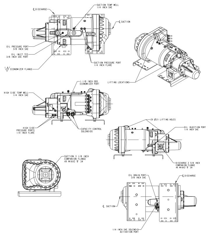
Fig. 1 - 06TS Compressor Physical Data and Connections
