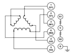
Fig. 32 — Terminal and Sensor Pin Layout
