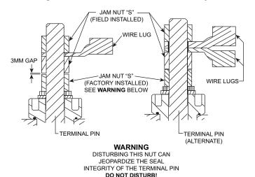
Fig. 33 — Terminal Pin Cross Section
