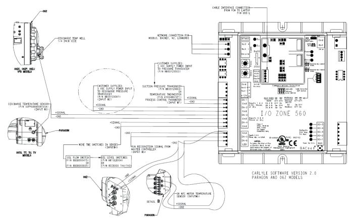
Fig. 25 — CCM Inputs, Version 2.0
