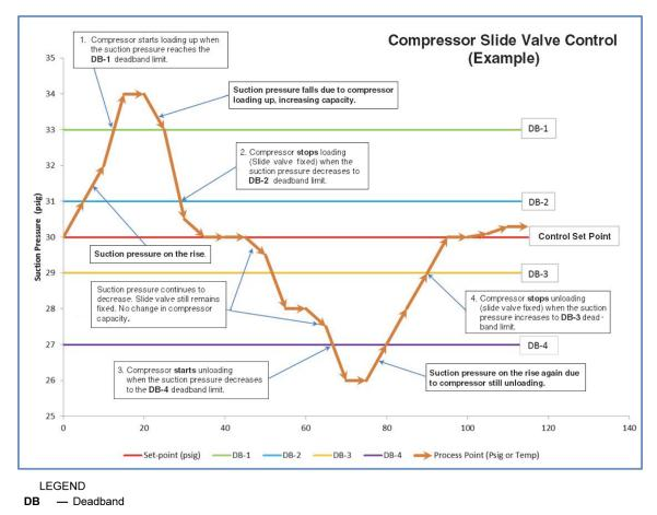
Fig. 27 — Paragon Slide Valve Control Illustration
