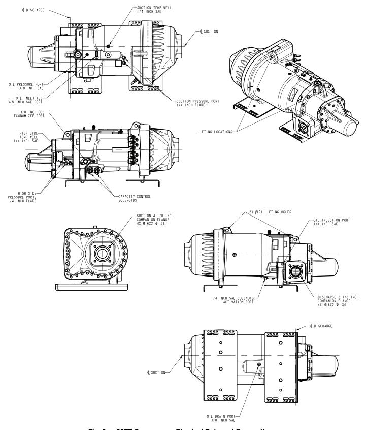
Fig. 2 — 06TT Compressor Physical Data and Connections
