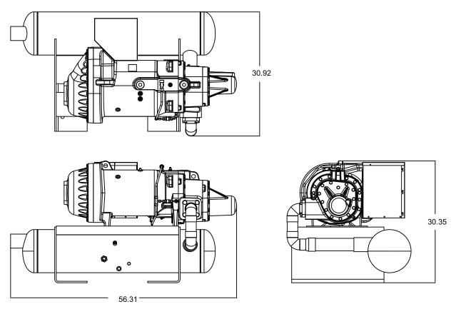
Fig. 37 — 06TSA186 Assembly Drawing
