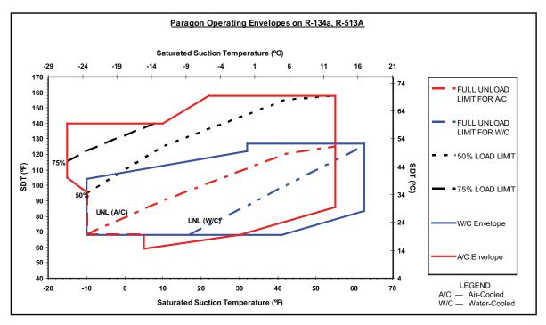
NOTE: Liquid injection may be required when operating fully unloaded. Contact Carlyle Applications Engineering for valve sizing requirements.
