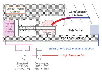
Fig. 21 — Configuration for Maintaining Part Load
