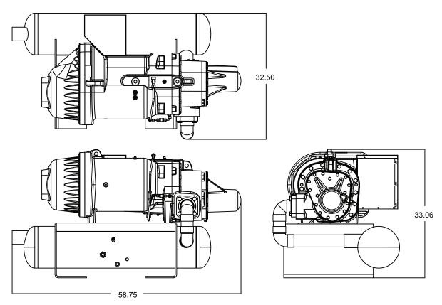
Fig. 39 — 06TTA301 Assembly Drawing
