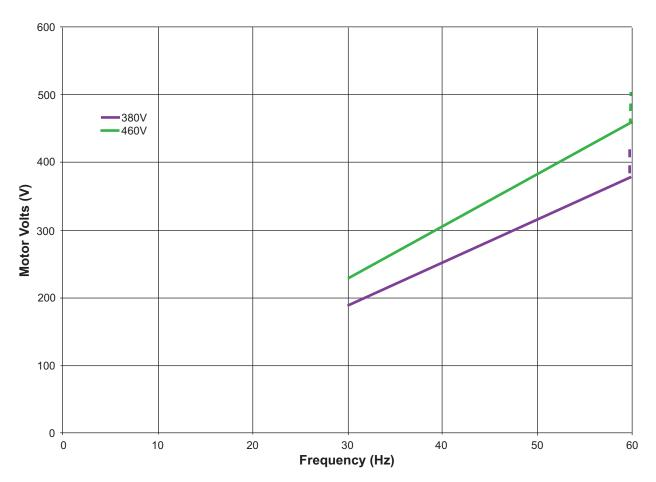
Fig. 31 — Sample Compressor Motor Voltage Curves
