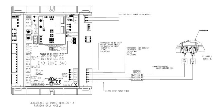
Fig. 24 — CCM Outputs, Version 1.5
