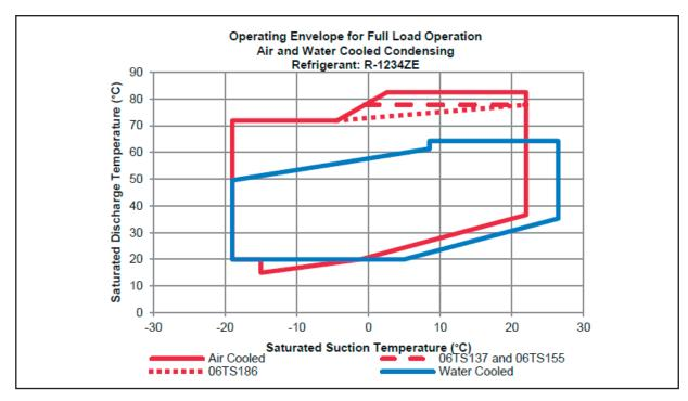
Fig. 5 — Operating Limits for Full Load Operation
