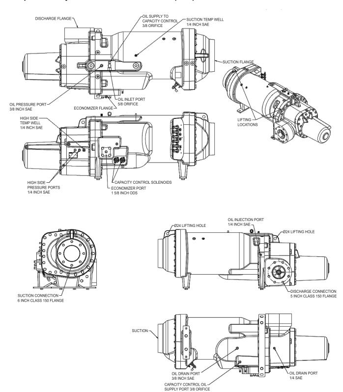
Fig. 4 — 6TV Compressor Physical Data and Connections
