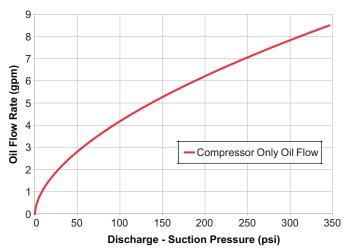
Fig. 16 — Oil Supply at Compressor
