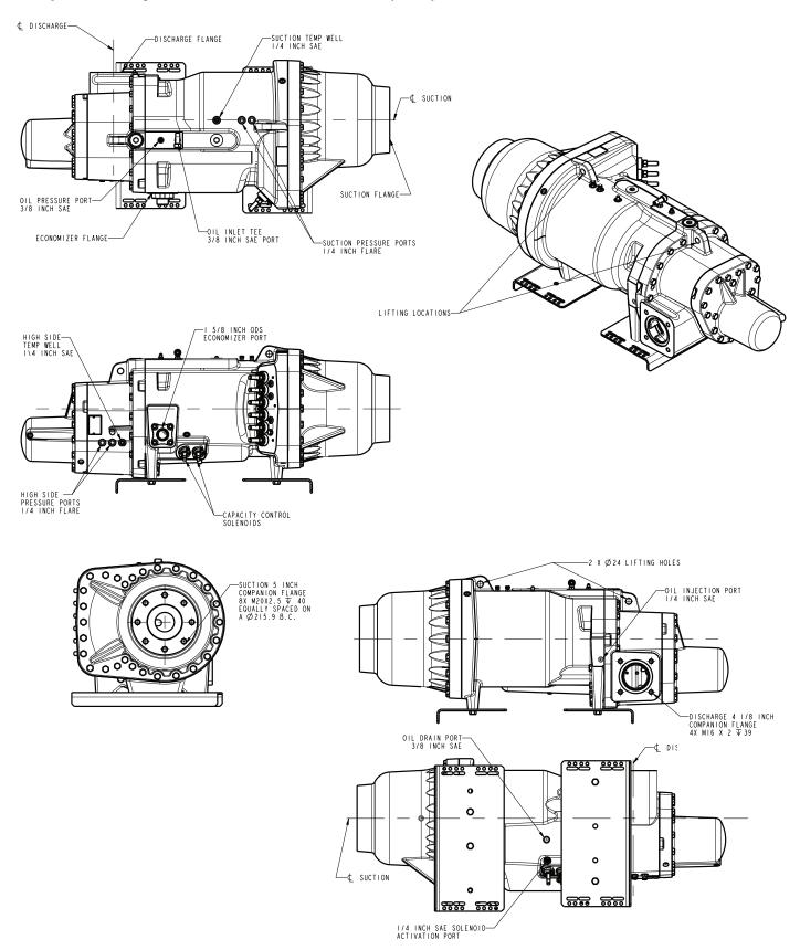
Fig. 3 — 06TU Compressor Physical Data and Connections
