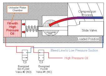
Fig. 19 — Fully Loaded Operation
