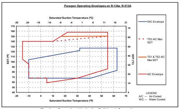
Fig. 6 — Operating Limits for Full Load Operation
