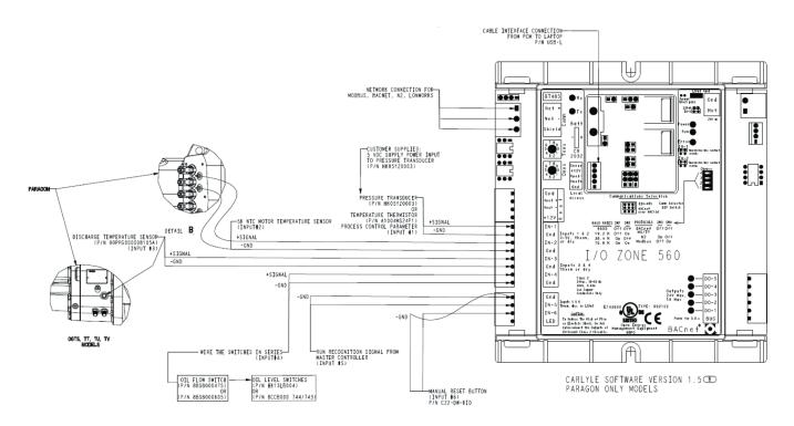
Fig. 23 — CCM Inputs, Version 1.5
