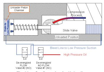
Fig. 20 — Configuration for Unloading
