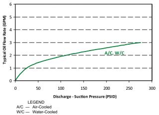
Fig. 10 — Oil Supply at Compressor
