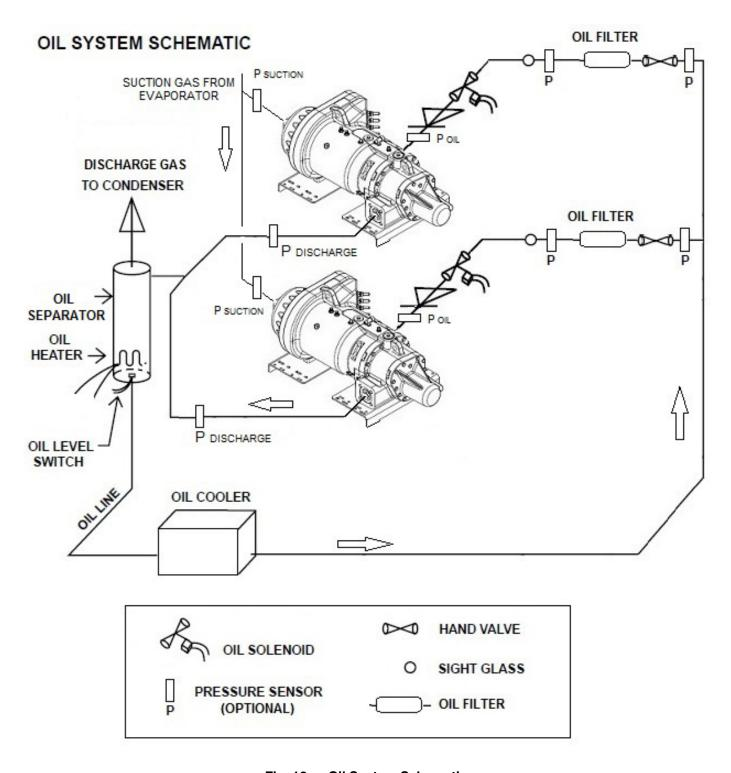
Fig. 18 — Oil System Schematic
