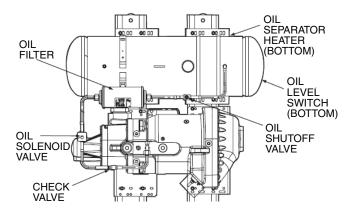
Fig. 9 — Oil Supply System Components
